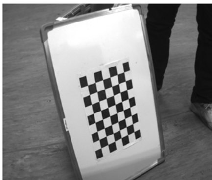
(a)左右摄像机棋盘图像样张 (a)Chessboard sample images acquired by two cameras
