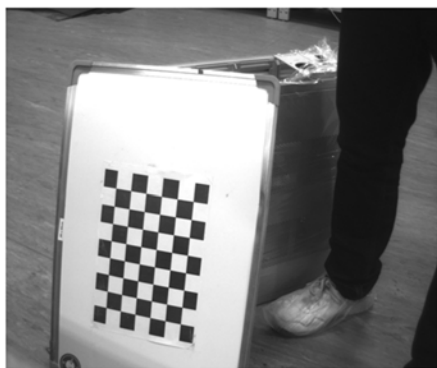
(a)左右摄像机棋盘图像样张 (a)Chessboard sample images acquired by two cameras
