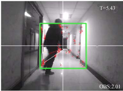
(b) 前方有障碍检测结果 (b) Detection results with obstacles in front
