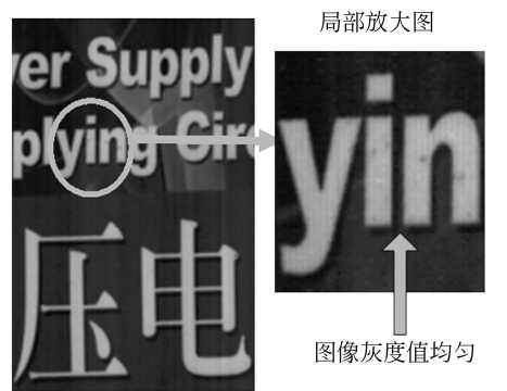
(b) 二次触发法扫描图像 (b) Scanning image with two-trigger method
