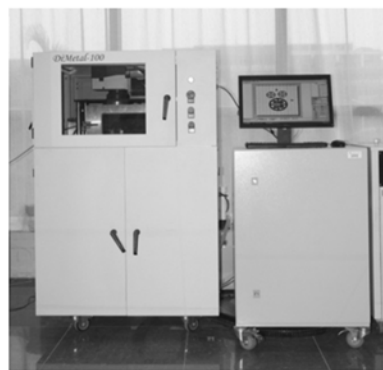
(b) SLM 设备 Dimetal100 (b) SLM equipment Dimetal-100
