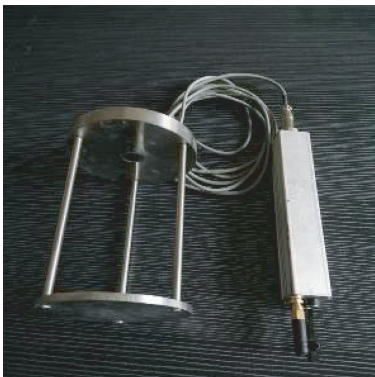
(b) 水下声速测量装置 (b) Underwater sound velocity measurement device
