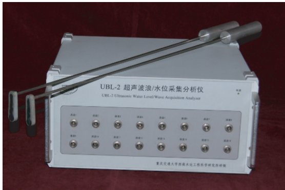
(a) 超声水位测量传感器、信号采集分析仪 (a) Ultrasonic water level measurement sensor and signal acquisition system
