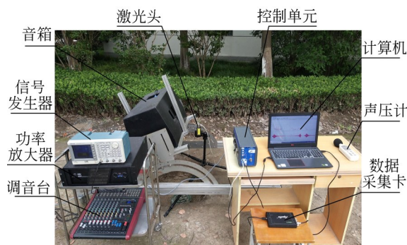
图 6 基于激光自混合测振的声共振探雷实验系统 Fig. 6 Experimental system of acoustic resonance landmine detection based on laser self-mixing vibration measurement
